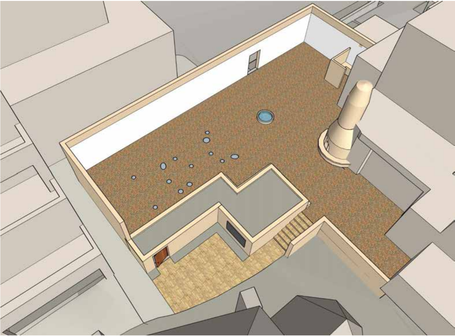
New enclosure wall and patio. Oculi provide glimpse to Boiler Room below.
